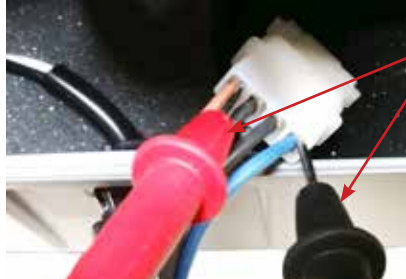
Testing Compressor Voltage
